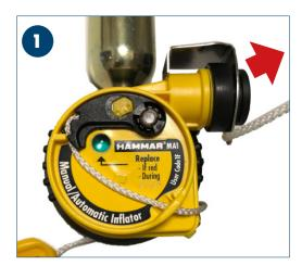
Dismount the conversion cap by puling the cord or push firmly on the metal part away from the valve.
